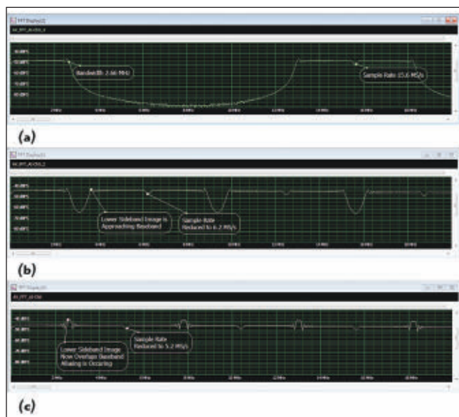
▲ Fig. 2 A frequency domain view of a sampled signal, where the sampling rate is well above the Nyquist frequency (a) and approaching the Nyquist frequency (b). Aliasing occurs when the sampling rate is below the Nyquist frequency (c).
