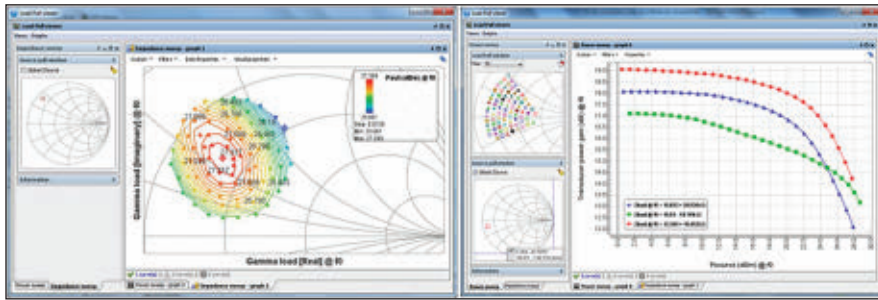
▲ Fig. 7 Load-pull iso-contours and gain compression curves under nonlinear operating conditions.
